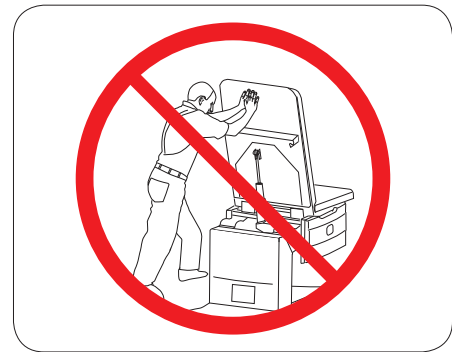
Figure 11. DO NOT Push on Backrest
