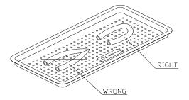
20. Packs should be placed upright on the tray. They should not be touching each other or the Chamber walls. There should be about 1" between packs for proper steam circulation.
