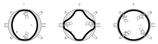
Pull off the gasket from the door groove. Install the new gasket as described in drawings 1, 2 and 3 above.
