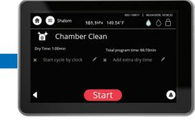
In order to efficiently clean the 8 autoclave chamber (once a week or every 25 cycles), choose "Chamber Clean" cycle and place a Chamber Clean tablet at the back of the chamber. Close the door and begin the cycle.
