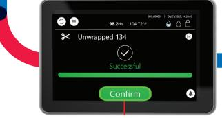
Once the sterilization cycle 6 is complete - press the "Confirm" button in order to open the door.
