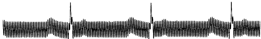
Regular AC Line Interference
